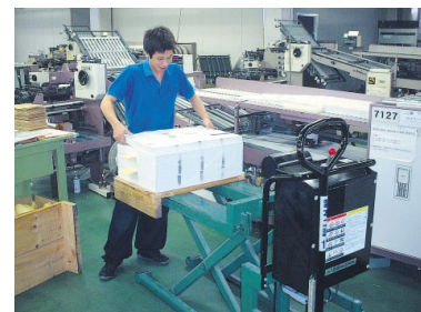
Match the height to machinery to match levels
