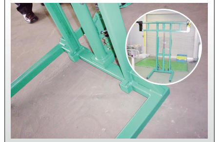
Fork (Legs) Width Extension [up to 1500mm]
