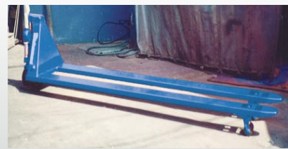
Fork Extensions (possible capacity reduction)
